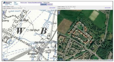
**Above**: Comparing old mine shafts on the Geological Survey maps (left) with present day satellite imagery (right) at Newtongrange
