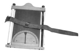
On the reverse is an inclinometer to measure angles of height.
